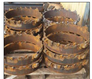
Pile drill teeth
